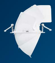
The entire face surface of the reflector moves outward, so that no light is spilled into the ceiling – no matter how far the angle is changed. This optimizes the light output for further energy savings, and it also allows for very precise fine-tuning of the accent lighting in the shop.
