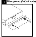
Attach filler panels to ends of housing using two supplied screws shown above.
