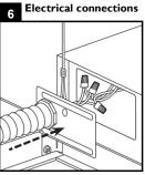
Make all electrical connections to the fixture.
