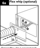
Optional Flex whip is prewired inside fixture. Remove packaging and insert snap-in fitting into wiring cover. Complete electrical connections at other end of whip in accordance with local building codes.
