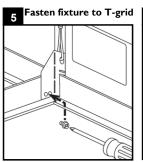
Use a #8x1/4" sheet metal screw to fasten fixture to T-grid and use a hanger wire to tie off appropriately in acodes (screws and hanger wires supplied by others.
