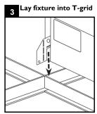
Lay fixture into T-grid.
