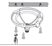
Surface Mounting/吸顶安装
