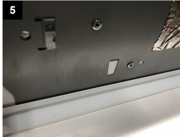
The housing should look as above image on joining ends. Ensure that the broken off sheet metal should not fall into the fixture.
