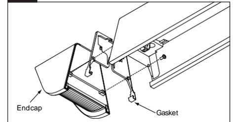
Snap on the gasket to the end of the fixture and attach end caps using supplied #8 screws.
