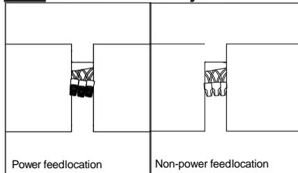
Complete power connections between fixtures.
