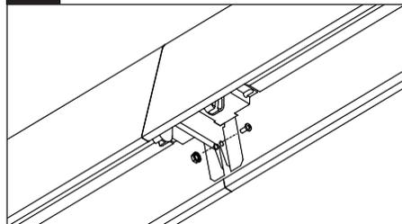
Join fixtures using supplied #8 screws and lock-nuts.
