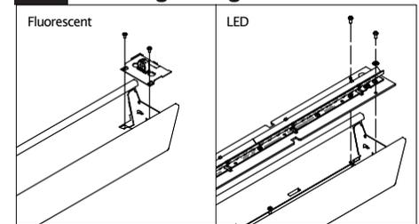
Remove socket saddle or LED light engine to gain access to mounting channel. When removing LED light engine be sure to disconnect the low voltage wire harness.
