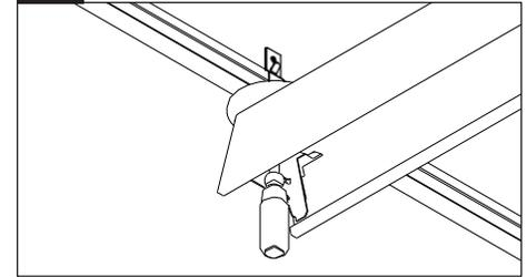
Using the supplied 1/4-20 nuts attach the fixture to the ceiling through the slots in the top of the fixture. DO NOT FULLY TIGHTEN. The mount should be able to slide, but be snug.
