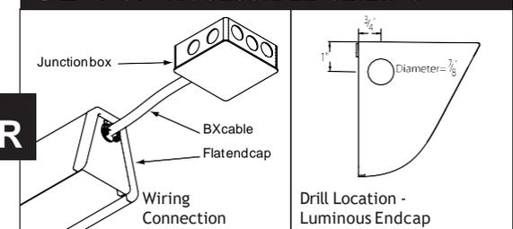
For non-accessible ceilings, drill 7/8 hole (location marked on Flat endcap: see diagram on right for drill location on Luminous endcap). Attach armored cable from the junction box (supplied by others) according to code.
