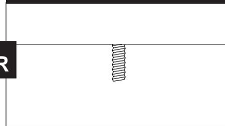
For non-accessible ceilings install 1/4 -20 stud extending 1/2 from ceiling. (see Mount Spacing Diagram on Page 1).
