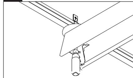
Tighten mounting bracket. Reinstall socket saddles or LED modules (remember to reconnect the low voltage wire harness). Install power plate and plug.
