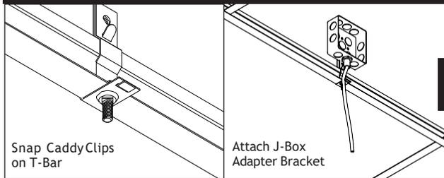
Snap caddy clips and 1/4 -20 threaded bolts on T-bar at specified mounting locations (caddy clips and 1/4 -20 threaded bolts supplied with mount kits). Tie-off caddy clips with guy wires (supplied by others) according to code.
