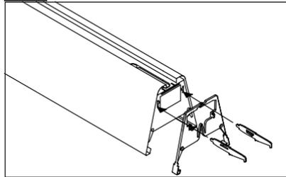
On the floor, slide variable mount bracket into next fixture in run. Attach joiner-aligner brackets, power plate and plug into opposite side.
