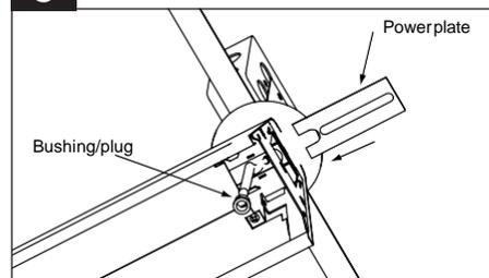
Slide power plates into fixture ends. Slide the supplied bushings over the SVT cord and snap into the power plate. If it is a non power location plug the hole with supplied plug bushing.
