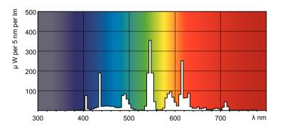
Spectral Power Distribution Colour - 24W/835 Min Bipin T5 HO ALTO UNP
