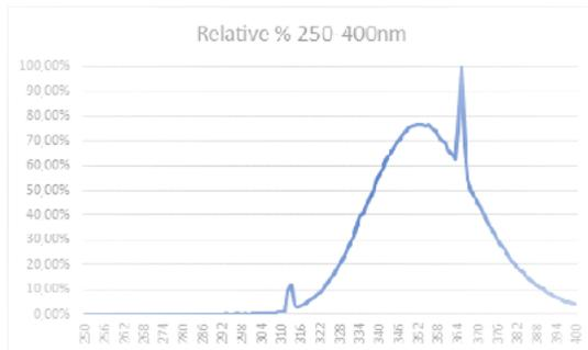
Spectral Power Distribution Colour - F71T12 UVA 100W
