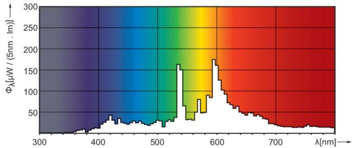
Spectral Power Distribution Colour - MASTERC CDM-R 70W/830 E27 PAR30L 40D 1CT
