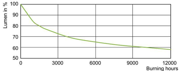
Lumen Maintenance Diagram - HPI-T 2000W/646 E40 220V CRP/4
