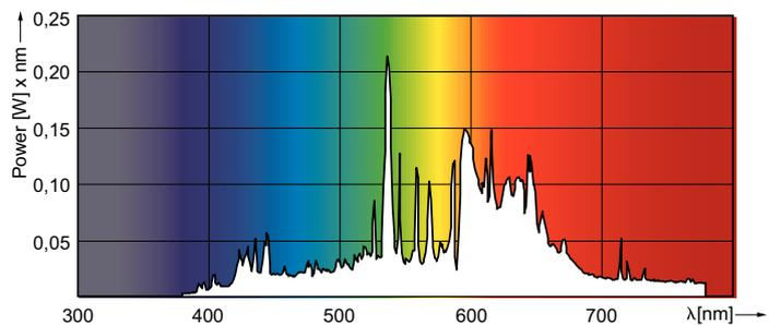
Spectral Power Distribution Colour - MC CDM-R Elite 70W/930 E27 PAR30L 10D
