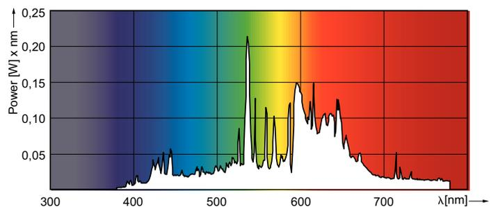
Spectral Power Distribution Colour - MC CDM-R Elite 70W/930 E27 PAR30L 40D
