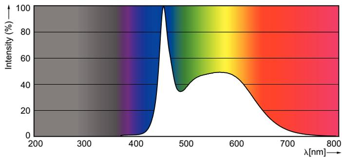
Spectral Power Distribution Colour - CorePro LEDtube 1200mm 18W 865
