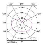
Light Distribution Diagram - BC10A19/AMB/927/DIM 120V
