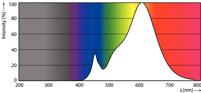
Spectral Power Distribution Colour - MAS LEDspot CLA ND 9-60W 827
