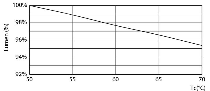
Lumen Maintenance Diagram - CorePro LEDtube 600mm 8W865
