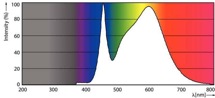
Spectral Power Distribution Colour - Master LED PAR30L 40W 30D 840
