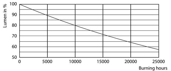
Lumen Maintenance Diagram - CorePro LEDspot 5-65W GU10 840 36D ND
