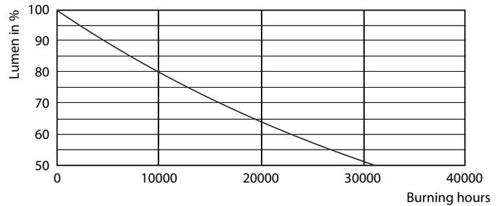
Lumen Maintenance Diagram - CLA LEDBulb ND 11-100W E27 CW A67 CL
