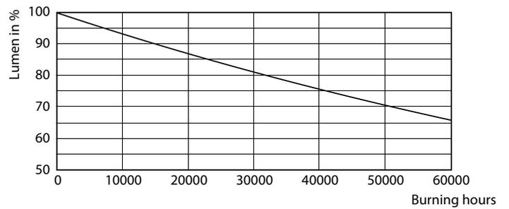
Lumen Maintenance Diagram - TForce LED HB MV ND 120-100W E40 840 WB
