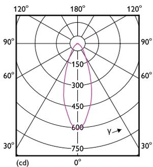
Light Distribution Diagram - LEDspotGU10EcoHome 50W 827 36D HV
