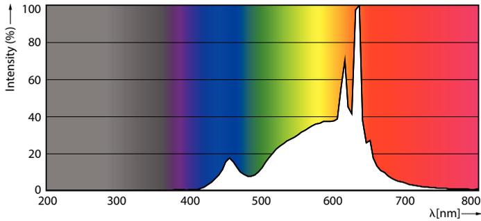
Spectral Power Distribution Colour - CorePro LEDbulb D 10.5-75W A60 E27 927
