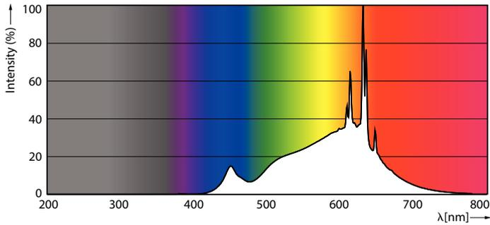
Spectral Power Distribution Colour - MAS LEDspot CLA D 13-100W 827 PAR38 25D
