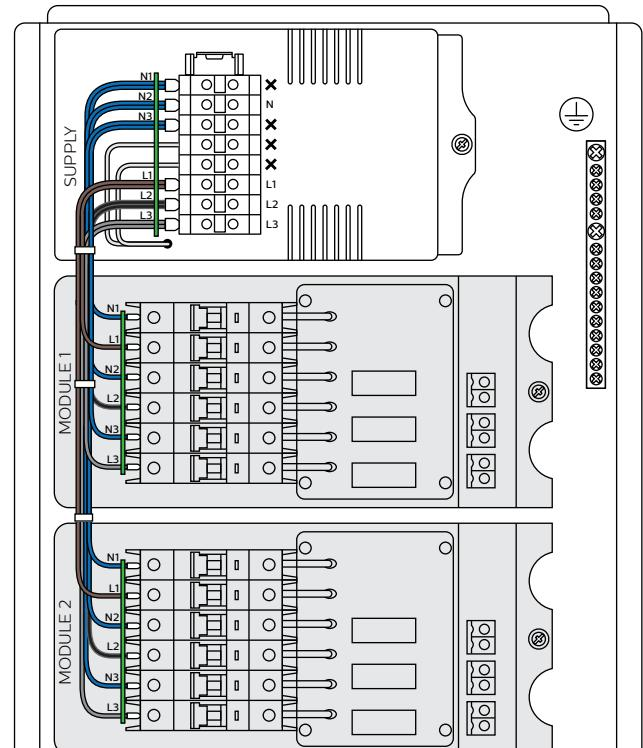
! Refer to enclosure label for earth bar wire gauge and torque ratings
