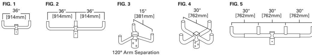
These steel pole brackets are used for mounting with 2" slipfitters on round or square steel poles. Poles must be specified with a simplex fitting and hardware which allows the bracket to be bolted direct to the fitting on the steel pole at the job site. Location of the bracket with respect to the base of the pole and the hand hole must be specified on the order for the pole. All brackets are finished with bronze paint.
