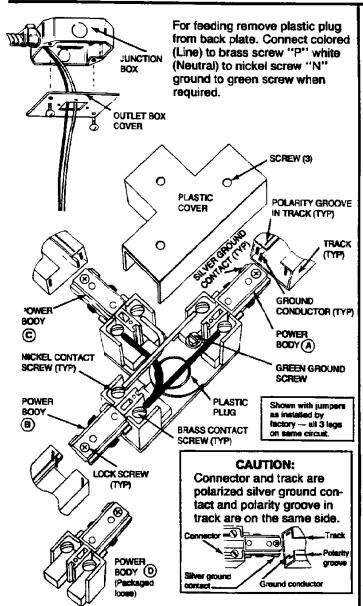
NOTE: Adjustable connector allows track to be powered at either end depending on installation requirements.
