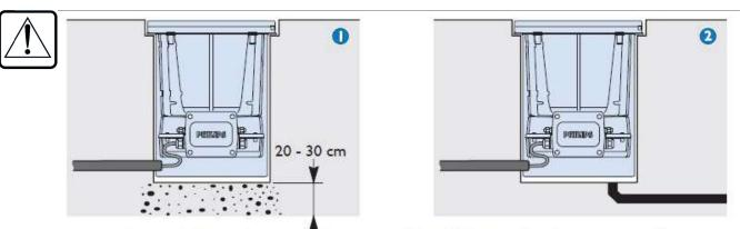
Prepare always 20 - 30 cm of drainage gravel and check that i works: fill the tube of water and check that it completely disappear within 30 min.lf it doesn't work study a further drainage system (2).
