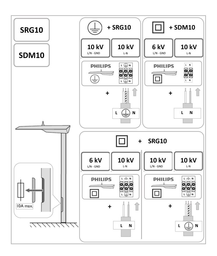
**EN (EN) 10kV extra surge protection (SRG10)** is ensuring Differential mode protection.
