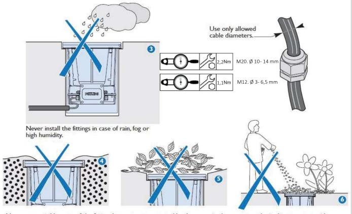
Never cover visible parts of the fitting. Any part not protected by the recessing box, must not be in direct contact with the ground or in contact with aggressive chemical elements (ex. fertilisers, herbicides, lime (6)).
