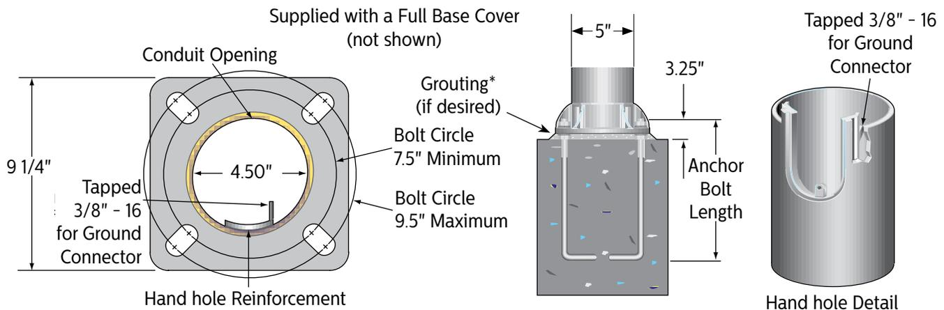
\* Grouting should include a drainage slot or tube (by others) to permit water to drain from the base of the pole. Failure to provide drainage may weaken the pole base structure over time and may result in pole base failure, for which Gardco is not responsible.
