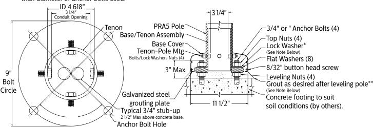
NOTE: Internal clearance of tenon/pole mounting bolts dictates allowable area for stub-ups.
