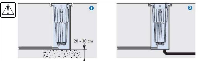
Prepare always 20 - 30 cm of drainage gravel and check that i works: fill the tube of water and check that it completely disappear within 30 min.lf it doesn't work study a further drainage system (2).
