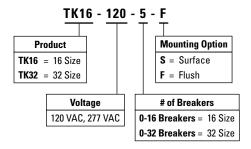
Example: TK16-120-14-F specifies a 16 circuit flush mount enclosure with 15 120V circuit breakers.
