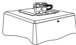
3. Slide fixture onto outlet box.
