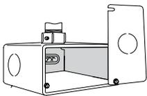
2. Install slide plate on top of ballast housing with three screws (provided).
