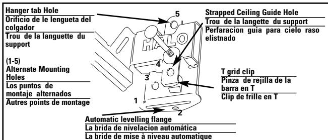
**Step 3.** Snap fixture on T-bars. Secure with screw (not included as shown (Fig. 4).
