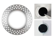
Mud-in ring (FMR): Low profile, non-metallic mudin ring provides a raised rib to plaster up to and a 3/16" flange thickness. The ring is attached to the ceiling material as opposed to the frame-in kit to avoid conduction of heat and vibration which can cause yellowing or cracking of the plaster.
