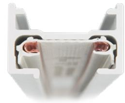
**Lightolier Basic Track** is a one circuit, one neutral track system designed to work with Lightolier track luminaires. The track can be installed individually, in straight runs, or in a variety of patterns to suit numerous applications. Lightolier track is field-cuttable and can be surface mounted, stem mounted, or installed in a recessed slot.
