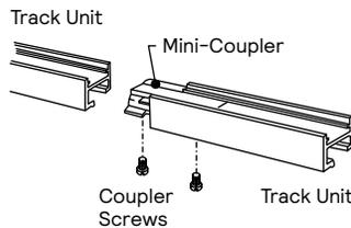
Used to connect two pieces of track together mechanically and electrically. Power can not be fed to Mini-Coupler.
