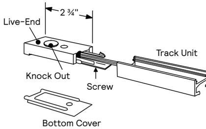
Knock out permits direct feed with electrical connector. Use with plain track.
