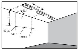
EXAMPLE: With track located 4' from wall and multiple units spaced 6' on center and aimed  $45^{\circ}$  from horizontal, the illumination on wall 4' from ceiling will be 59 f.c. beneath units and 54 f.c. between units.
