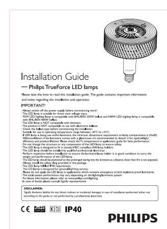
For replacing MH HID lamp, convert to mains voltage input Warning sticker Perform a visual inspection to ensure the lamp-holder and internal wiring is not damaged, if the lamp-holder is damaged, corroded, charred, blackened, or loose, the lamp holder should be replaced with new lamp-holder if the internal wire is damaged, it should be replaced with new wire. I) Switch off the power to luminaire. Remove diffuser/glass (if provided) and existing lamp from the luminaire.
