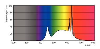
Spectral Power Distribution Colour - MC LEDspot IA 4.7-50W GU10 940 36D
