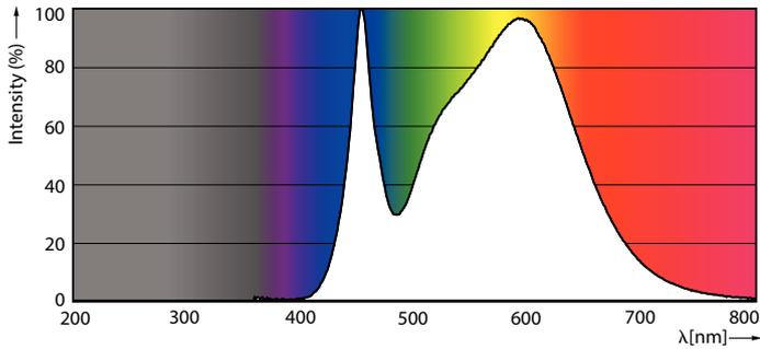
Spectral Power Distribution Colour - TForce Core HB MV ND 30W E27 840 G3
