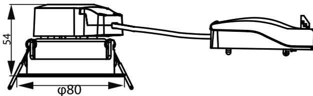
Cut-out hole diameter - Ø68mm
