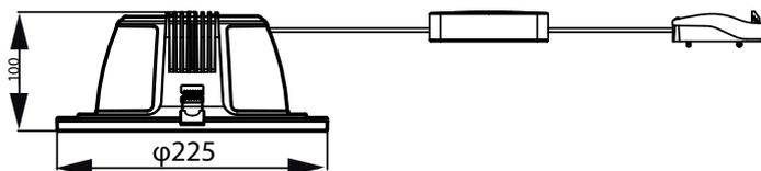
Cut-out hole diameter - Ø200mm
