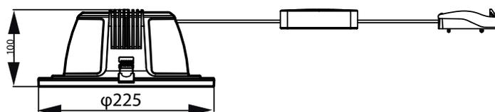
Cut-out hole diameter - Ø200mm
