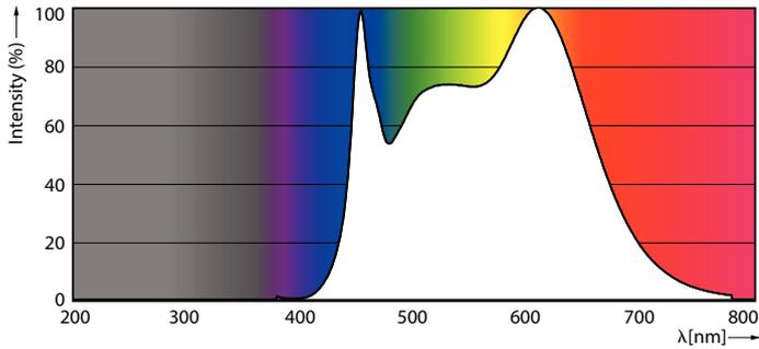
Spectral Power Distribution Colour - MAS LEDspot VLE D 9.5-75W 940 PAR30S 25D
