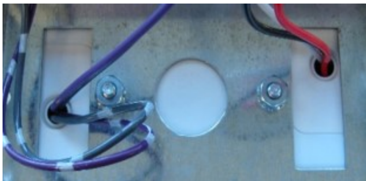
SR Bridge (SRB-BS) may be mounted on the cover plate of above metal box with proper slots for mounting screws and wires.
