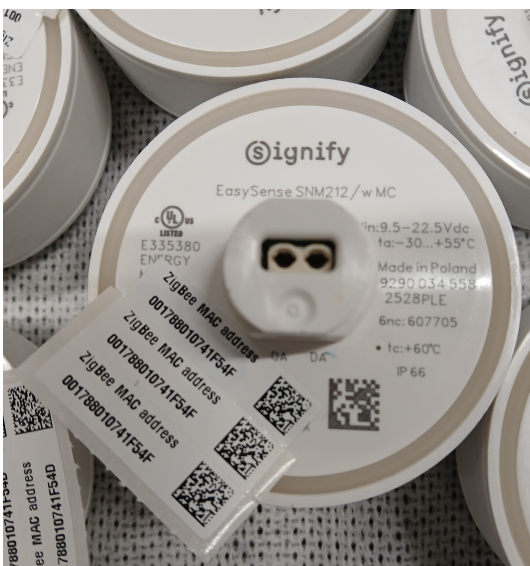
Labels with unique Zigbee Mac address
