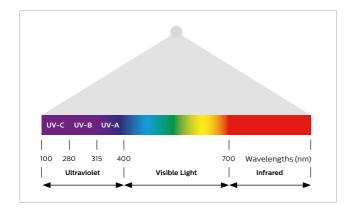
Wavelengths in the photobiological ultraviolet spectral band known as UV-C have been shown to inactivate bacteria, spores and viruses. The peak output of Philips germicidal lamps (253.7nm) is close (80-85%) to the maximum effectiveness of UV-C (265 nm).
