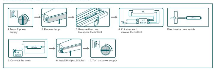
To check if your ballast is compatible, always refer to the latest update of the Philips LEDtube compatibility on www.philips.com/ledtube
