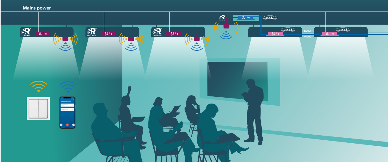
Figure 6: Using existing wired DALI luminaires? Simple. Add them into the network at any time using an SR bridge.
