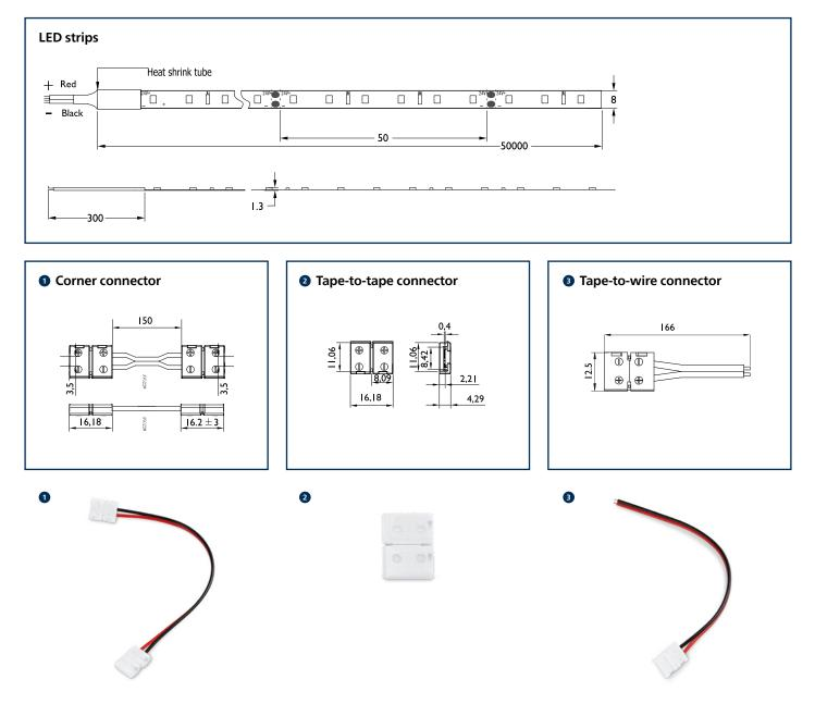
**Attention:** when using connectors please take the maximum tape length into account. Never exceed 2A or 48W for a series connection. Detailed information can be found in the installation manual.
