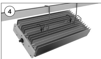
Hold the module firmly with two hands and position both V-shaped parts of bracket (A) over both hooks of bracket (B). /
