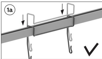
Hook on bracket (B) to the C-profile by pressing in the direction as depicted by the 2 arrows in Fig.1a. Make sure that bracket (B) is firmly enclosing the profile, by assuring that the wire is clamped underneath the profile. Bracket (B) is used as an example, the same way of working holds for types (C) and (D). /
