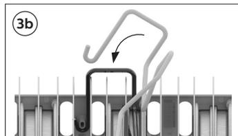
Move the bracket downwards, from vertical to horizontal position. Firmly press the end of the bracket towards the mounting feature shown in Fig.3b. Make sure the hook is firmly clamped underneath the mounting feature. /
