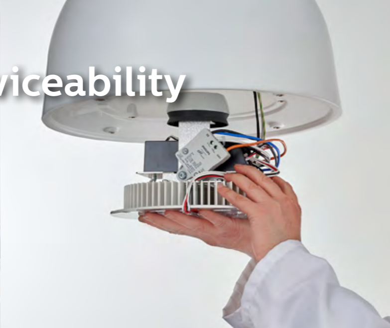
The Copenhagen2 family is easy to maintain. Simply remove front glass and disconnect the LED unit for replacement
